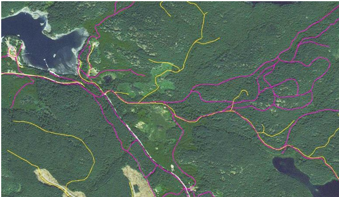
Figure 8. Overlapping and offset roads on Quadra Island from two different data layers: provincial forest tenure resource roads (yellow) and provincial digital road atlas roads (purple).
