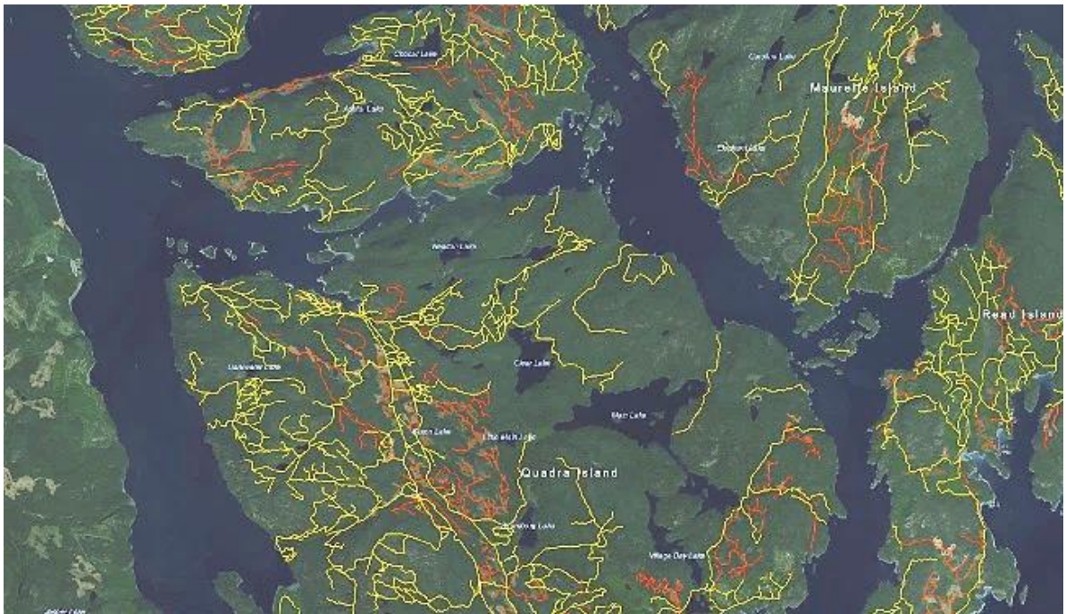
Figure 7. Missing roads digitised (in red) from satellite imagery
